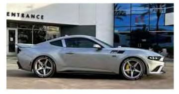
On the outside, the 2024 Saleen 302 White Label utilizes a host of upgrades designed to maximize airflow, starting up front with a totally new front fascia that features an aerodynamic splitter and an air damn designed to generate large amounts of downforce for cornering performance. From there, the new White Label features a revised hood vent to make it easier for hot air to escape the engine bay, along with a new axial grille and a rear wing.
